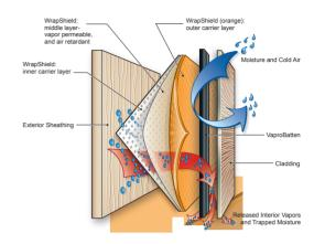
WrapShield IT WRB/Air Barrier is vapor open, allowing trapped moisture to escape and air tight preventing costly air migration.
