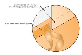
Clear integrated horizontal tape and pre-marked lap template increase installation accuracy and ensure shingled overlap.
