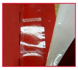
Ensure correct alignment, using the dotted line at the vertical seam, prior to removing release paper.
